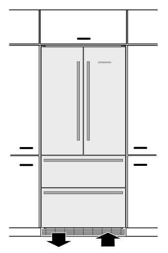
It is important to use the provided cover grille for the ventilation opening. This opening must not be covered with a cabinet base.
